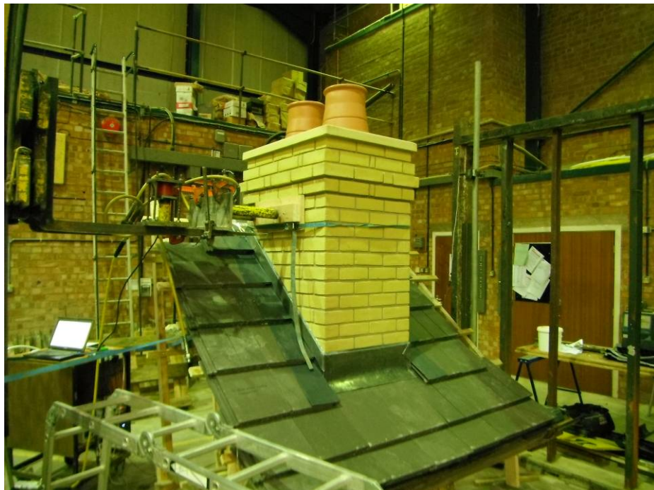
Plate 2: Mono Pitch Chimney under UDL
