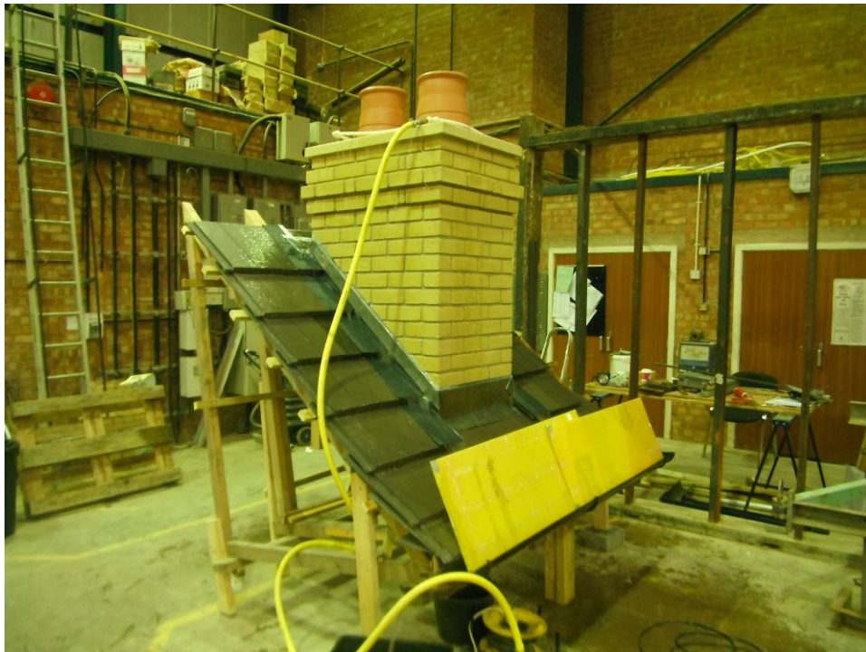
Plate 5: Mono Pitch Chimney under Soak Coat Water Test
