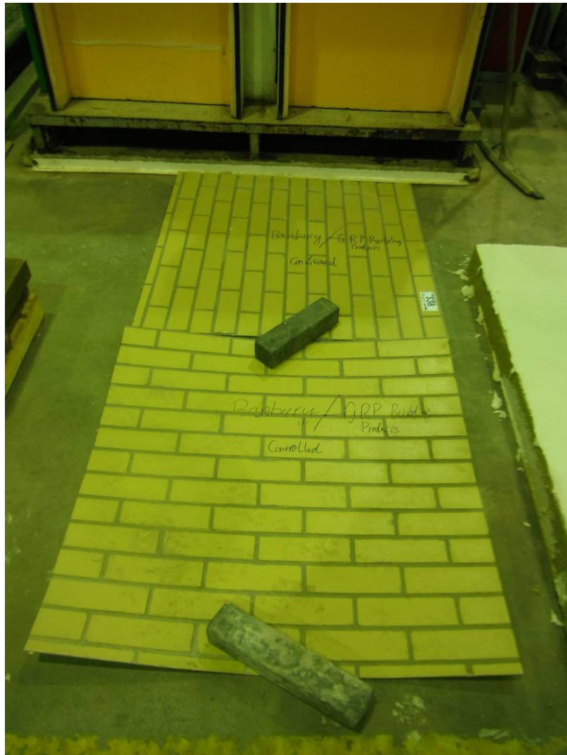
Plate 7: GRP Control Panel and Conditioning Panel after Accelerated Weathering Test
