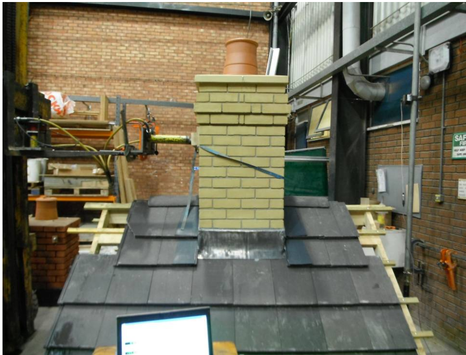
Plate 1: Mid Ridge Chimney under UDL
