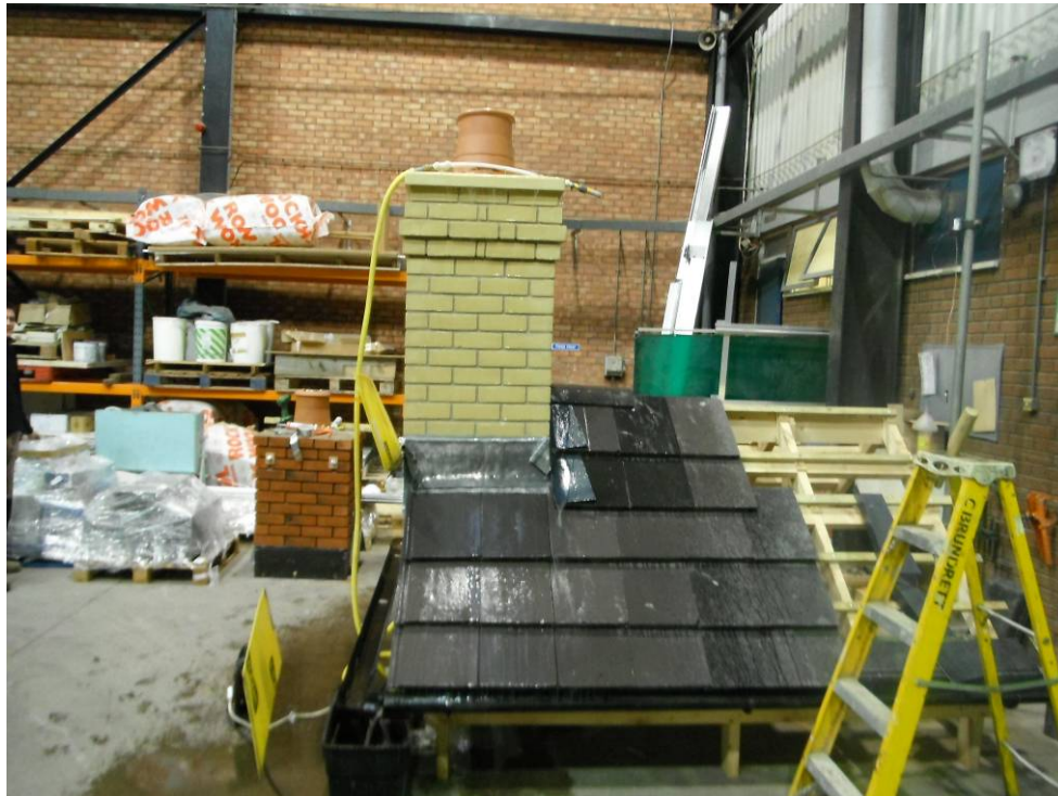
Plate 6: Gable End Chimney under Soak Coat Water Test
